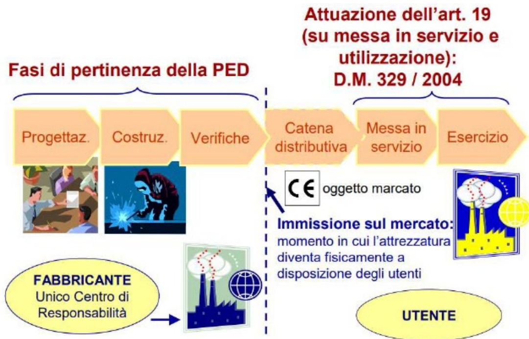
Figura 6 - Flusso processo algoritmo PED (Pressure Equipment Directive) [3]
